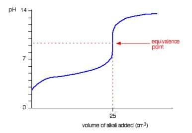
The start of the graph shows a relatively rapid rise in pH but this slows down as a buffer solution containing ethanoic acid and sodium ethanoate is produced. Beyond the equivalence point (when the sodium hydroxide is in excess) the curve is just the same as that end of the HCI - NaOH graph.
