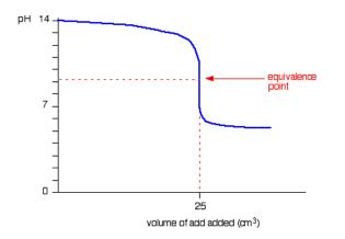
Past the equivalence point you have a buffer solution containing sodium ethanoate and ethanoic acid. This resists any large fall in pH.
