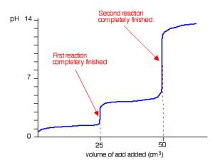
The curve is for the reaction between sodium hydroxide and ethanedioic acid solutions of equal concentrations.
