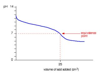
Notice that there isn't any steep bit on this graph. Instead, there is just what is known as a "point of inflexion". That lack of a steep bit means that it is difficult to do a titration of a weak acid against a weak base.
